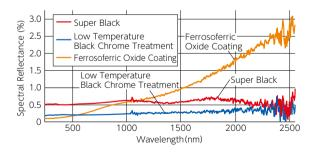
Low temperature black chrome treatment and super black result in extremely low spectral reflectance, which is optimal for optical instruments that require diffuse reflection prevention.
