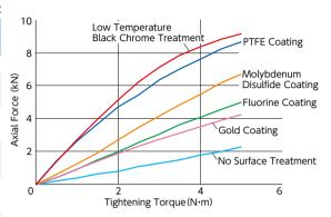
Test piece : Stainless Steel Socket Head Cap Screw M5 $\times$ 25 Strength Class : A2 - 70
