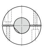
🔼 If the D-cut surface or key groove is not in the recommended position, the clamp part may be damaged if excessive load is applied due to hexagon socket head cap screw tightening.
