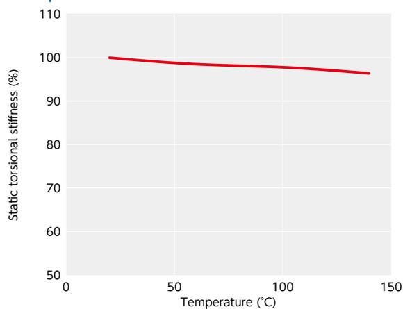
This is a value under the condition where the static torsional stiffness at 20°C is 100%.
