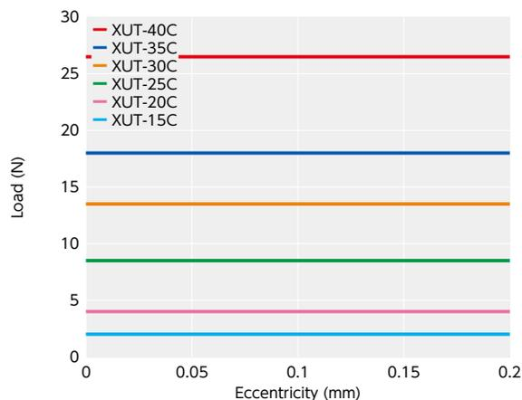
**XUT-C** has small eccentric reaction force and an extremely small shaft load generated by misalignment. This reduces the load to such components as shaft bearings.
