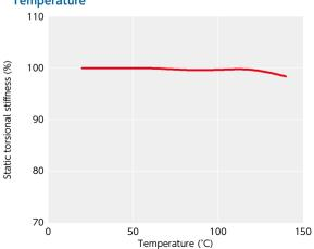
This is a value under the condition where the static torsional stiffness at  $20^{\circ}$ C is 100%.
