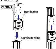
Push the CUTB-U button, and insert onto the T-slot in the aluminum frame in the unlocked state.
