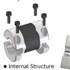
The designed shape of vibration-absorbing rubber achieves high torsional stiffness and high torque according to the finite element method. This product also succeeds in elongating its life by evenly dispersing the stress focusing on around the inner diameter of the jaw throughout the entire jaw.
