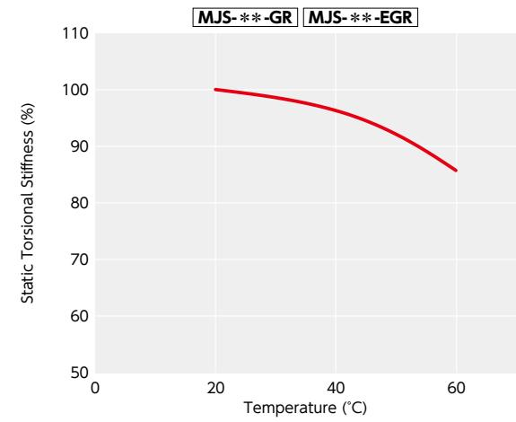
This is a value under the condition where the static torsional stiffness at 20°C is 100%.
