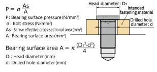
Head Diameter and Screw Effective Cross-Sectional Area
