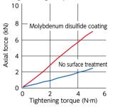
• Reference data for Hex Socket Head Cap Screw - Molybdenum Disulfide Coating **SNSS-M5-25-MO**.
