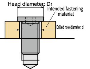
Head Diameter and Screw Effective Cross-Sectional Area
