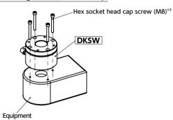
In order to pass the hex socket head cap screws (M8)\*3 through from above, align the rotating part through-hole and the main body counterbored hole phases with the clamp lever loosened. After aligning the phases, tighten the clamp lever and lock the rotation. Fix **DKSW** to the equipment with 4 hex socket head cap screws (M8)\*3.
