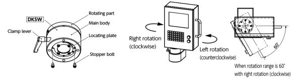
The control panel rotation angle can be restricted through a combination of the mounting position of the provided stopper bolts and the position of the locating plate.\*2
