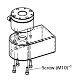
Fix **DKSW** with 4 screws (M10)\*3.
