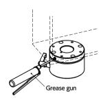
4 Insert at least 5.5cc of grease\*3 with a grease
