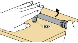
\*1: When the edge does not bite in and slipping occurs, remove SKEK using a socket wrench, and tap it lightly with a plastic hammer until it bites into a hex head bolt, hex nut, etc. Hitting with a hammer will transmit the impact to the part where the screw is attached. Be sure to pay attention to the place of use.
