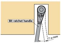
If there is space for the bit ratchet handle to rotate 7° or more, the screw can be turned continuously.
