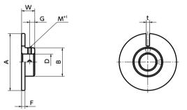
\*1: In a case where the bore diameter is  $\phi$  4 or less, the set screw is used in only one place.
