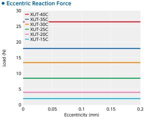
**XUT-C** has small eccentric reaction force and an extremely small shaft load generated by misalignment. This reduces the load to such components as shaft bearings.
