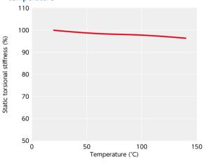
This is a value under the condition where the static torsional stiffness at 20°C is 100%. The change of **XUT-C** in torsional stiffness due to temperature is small and the change in responsiveness is extremely small. If the unit is used under higher temperature, be careful about misalignment due to elongation or deflection of the shaft associated with thermal expansion.
