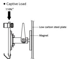
\*1: Captive load is a test value with stable static load. With the magnet securely attached to the material surface of a 10 mm thick low carbon steel plate under room temperature, load was applied from above, and the load at which the magnet separated from the material surface was measured.
