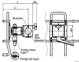
\*1: The clamp lever setscrews for the clamp lever type  $\boxed{\textbf{DTS}}$ have been changed from hex sockets to hexalobular sockets.
