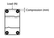
This is the force generated when compressing **XGT XGL XGS** in the axial direction. As the thrust reaction force becomes smaller, the force acting on the motor also becomes smaller.
