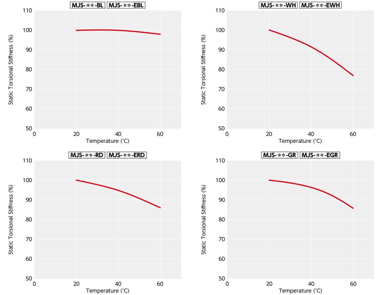
This is a value under the condition where the static torsional stiffness at 20°C is 100%. The change of torsional stiffness within the range of allowable operating temperature is as shown in the graph. Before using the unit, be aware of the deterioration of responsiveness.
