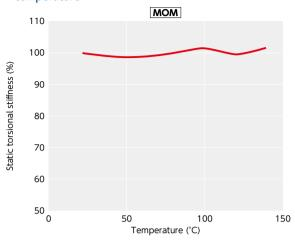
This is a value under the condition where the static torsional stiffness at 20°C is 100%. The change of **MOM** in torsional stiffness due to temperature is small and the change in responsiveness is extremely small.
