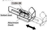
The use of a mechanism to fix the slotted steel and move **CUSH-2B** and the attachment to the desired position for fixing is also possible.
