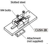
While continuing to push the button, move CUSH-2B to the location it should be fixed.
